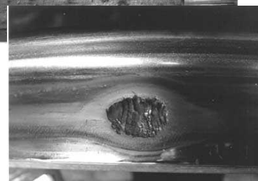
Figure 6: Wheel tread shelling
