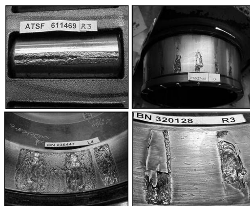
Figure 21: High risk bearing defects
